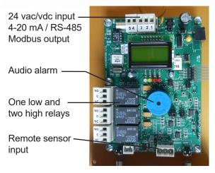
Plug-in connectors and easy access sensors for fast maintenance.
