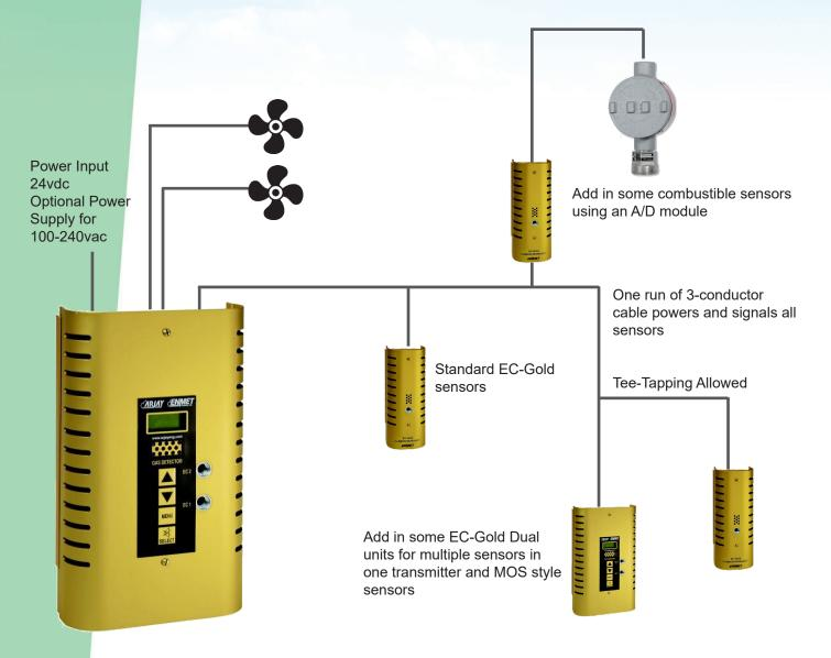
Mix and match: carbon monoxide, nitrogen dioxide, oxygen, ammonia, propane, hydrogen and more
